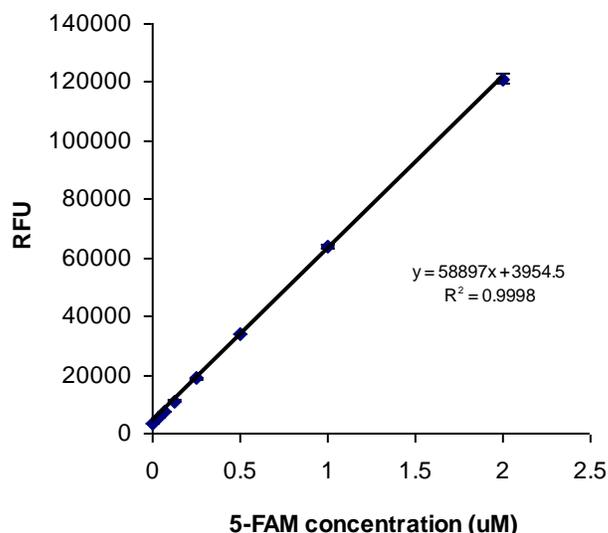
Figure 2. 5-FAM reference standard, 5-FAM was serially diluted in assay buffer containing substrate, and the fluorescence was recorded at Ex/Em=485 $\pm$ 20 nm/ 528 $\pm$ 20 nm. (Flexstation 384II, Molecular Devices)
